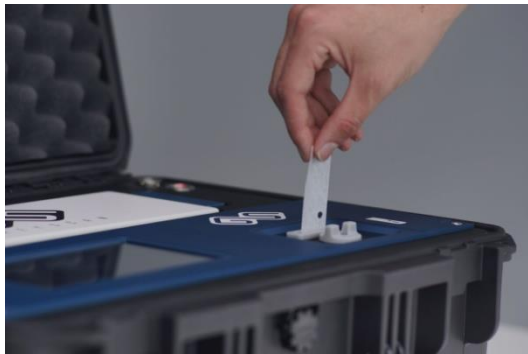
Figure 2: Insertion of a sample trap containing explosive residues into a CZE device
