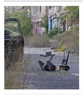
SUGV is a portable, single-person-lift robot with dexterous manipulation, providing dismounted EOD technicians and other responders with a highly mobile robot that climbs stairs and manipulates objects.
